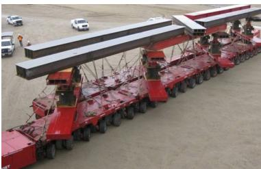
Example of a Self-Propelled Modular Transporters (SPMT)
